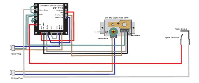
Electronic Burner Control CE12U AGA6953 Tandem Valve SIT 836 Wiring Layout Pilot – Low Flame – High Flame
